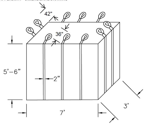
NOTE: All straps to be run/stitched completely under and around bag.
